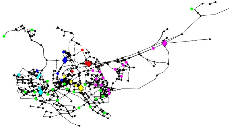
Figure 2 – Results for the localization of contamination sources with a time horizon of 24 hours.
