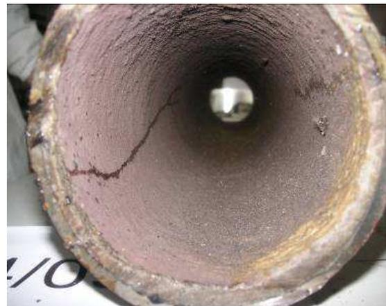
**Fig. 2: Cement coating with deposit**
