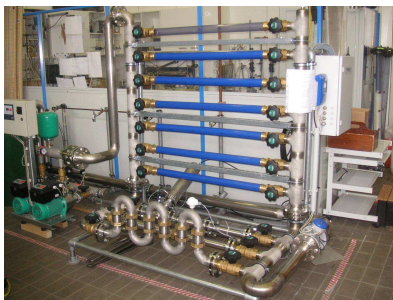
Fig. 2: Pilot test system used for the generation of drinking water biofilms on pipes and test coupons
